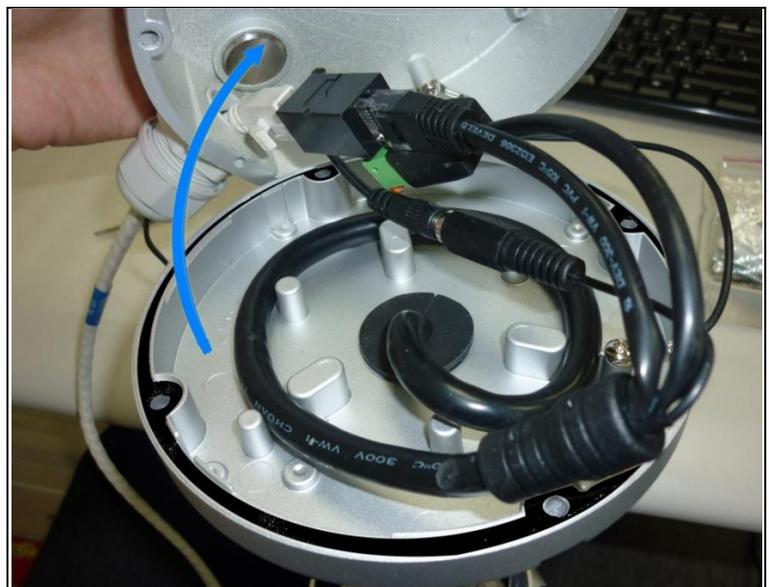
24. Finally, lock the screws on the lid, and leave no gap between lid and box bottom. Installation Finishes.
