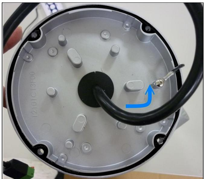
22. There lid design can fix the cable in order to prevent the cable from loose.
