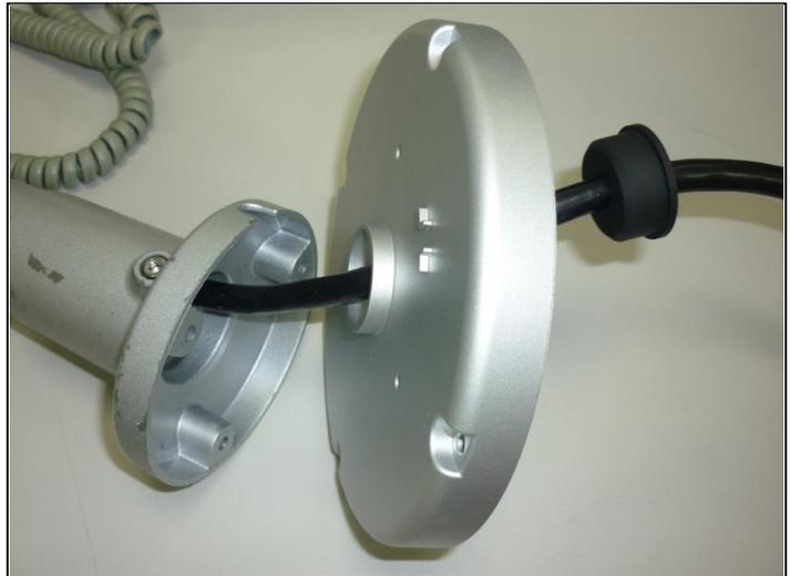
14. Flip down the box lid, and push the waterproof plug into the top hole until it fully fills the hole.
