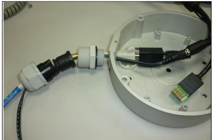
Ex. There's a rubber ring in the waterproof connector. If it's difficult to make the cable through the ring, you can cut ring.
