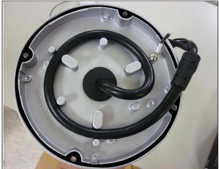
23. Take the box lid with coiled cables and cover it onto the box bottom. Before you close the box, make sure the black rubber ring on the fringe of lid is flat and sticks completely on the lid.
