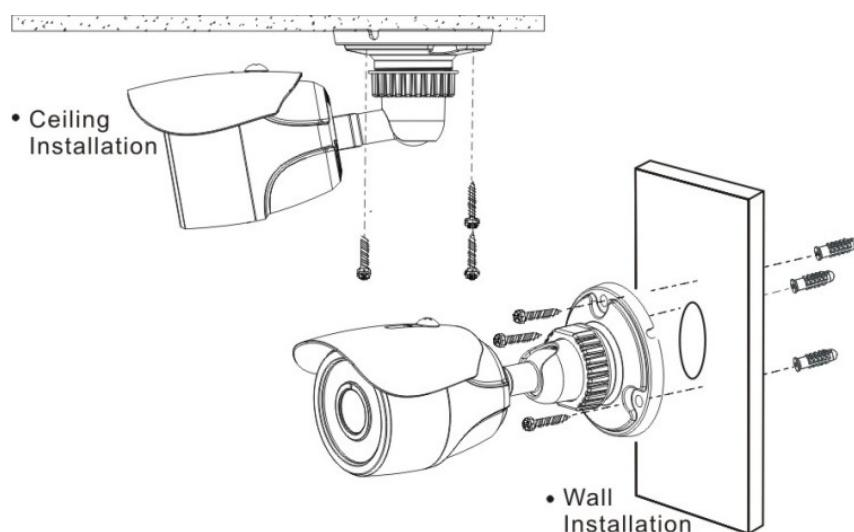
**Hint :** Make sure that the underside of the bracket is flush with the surface to seal it against outside influences.
