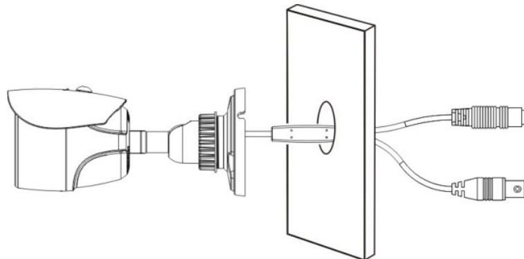
Use the included screws and dowels to fix the camera.
