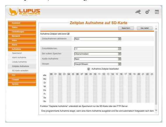
In addition to motion-controlled recording, you can also activate time-controlled recording. This can be made only to an SD card or an FTP server.
