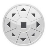
Use the arrows to control the camera simply by clicking the mouse. Click the square in the middle to move the camera automatically into the central position.
