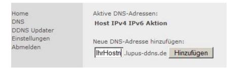
**Note:** To be able to access the camera with this host name via the internet, you need to set up port forwarding (NAT) on the router configuration page. In this menu, you can specify an arbitrary "public port" (e.g. 10000), the IP address of the camera (e.g. 192.168.178.20) as well as the "internal port" of the camera (e.g. 88).
