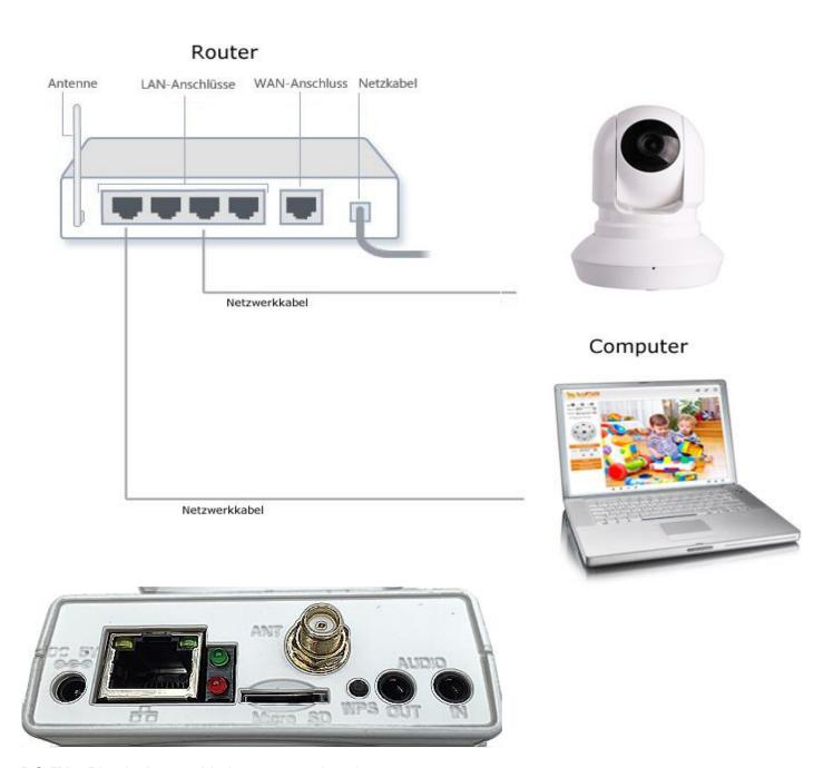
**DC 5V** – Plug in the provided power supply unit.
