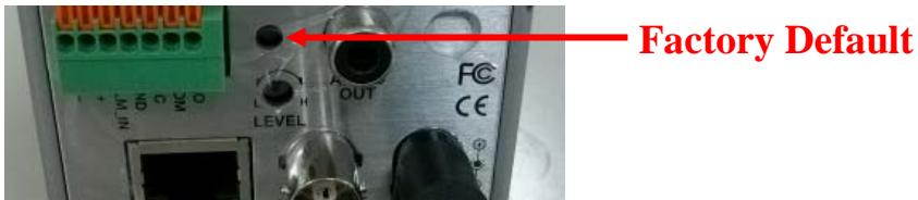
7. Plug in the power adapter and do not release the button during the IP Camera booting.
